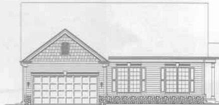
ELEVATION # 5 W/ SIDING w/ STONE WAINSCOT
