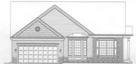
ELEVATION # 4 W/ SIDING & STONE VENEER
