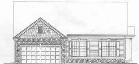
ELEVATION # 5 W/ SIDING & STONE VENEER
