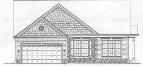
ELEVATION # 3 W/ SIDING & STONE VENEER
