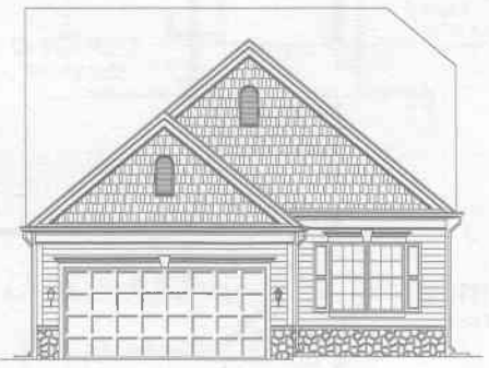
ELEVATION #2 w/ SIDING & STONE WAINSCOT (COVER)
