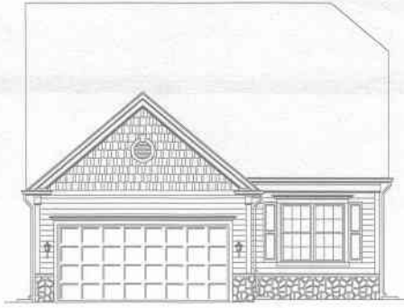
ELEVATION #1 w/ SIDING & STONE WAINSCOT
